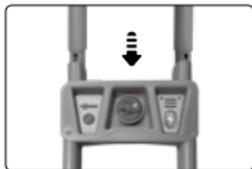
2. Insert two **Screws** on each side of the **Handle** and use a screwdriver to secure.
