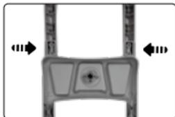
3. Insert the **Wheels** on both sides of the mower's body and press them in firmly.
